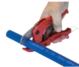
Cut pipe to length with pipe cutters for a clean swarf free finish.
