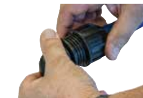
Firmly hand tighten the nut to the back stop. Check witness mark.
