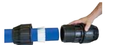
Loosen the nut and grip ring off the fitting and assemble onto the pipe a distance about 2x the pipe diameter.
