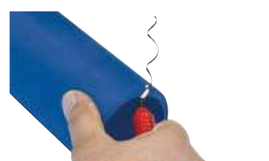
Use chamfer tool to remove sharp edge off the pipe and facilitate insertion through the O-Ring.
