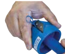
Use chamfer tool to remove sharp edge off the pipe and facilitate insertion through the O-Ring.
