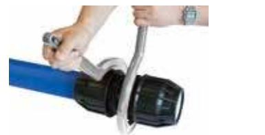
For sizes 75 -110mm use two nut wrenches to tighten the nut. Nut should be firmly tightened, but does not need to actually meet the external stop.
