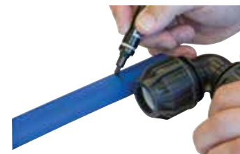
Witness mark the insertion depth.
