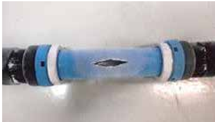
Photo of test at minus 30°C with NBR seals. Pipe bursts at 243.2 bar pressure but no failure of the fittings.
