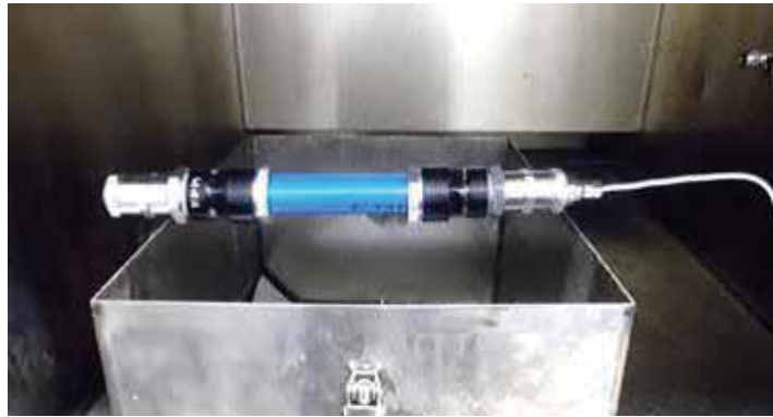
Photo of test at 535 bar. Pipe bursts but no failure of the fittings.
