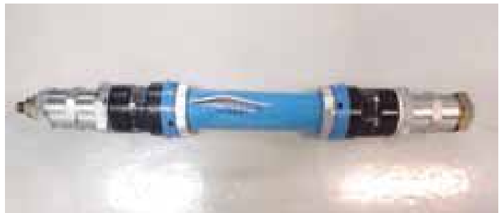
Photo of test at +100°C with NBR seals. Pipe bursts at 202.9 bar pressure but no failure of the fittings.
