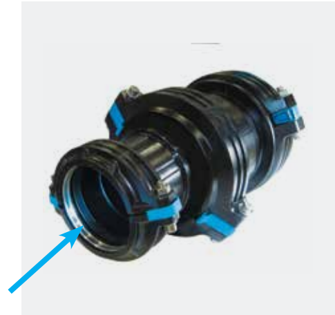
Insert the Reducer in the desired position, reassemble the clamp halves and tighten the bolts and nuts at a torque value of 15N/m.
