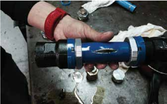
Photo of test showing high pressure pipe split at 535 bar, but still no failure of the fittings. The high-pressure test pump had to be pushed beyond its limits to finally achieve a burst point on this 70 bar rated pipe.
